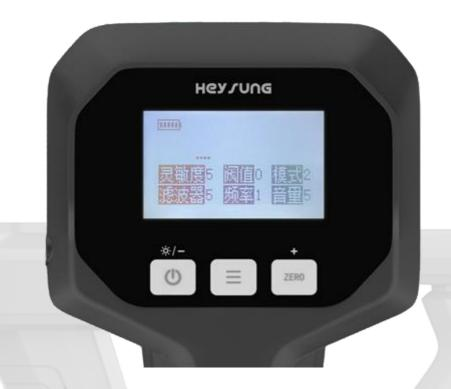
The controller of the HS-6000 portable pulse detector has three buttons, namely the power button, the menu button "MENU", and the zero adjustment button "ZERO".
